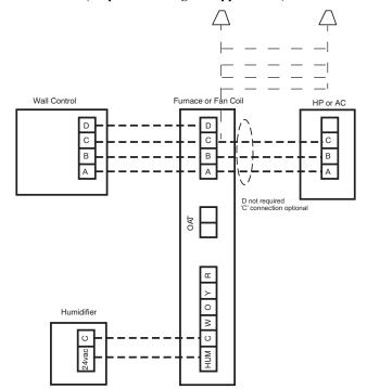
Fig. 5 – Infinity Furnace or Fan Coil Wiring with Communicating Variable Speed HP
