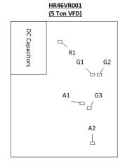
Fig. 28 – VFD LED Indicators
