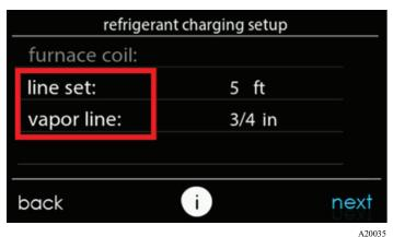
Fig. 17 – Select Line Set Length & Vapor Line Diameter
