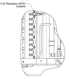
Fig. 30 – Outdoor Coil Thermistor Mounted on Coil Suction Thermistor (OST)
