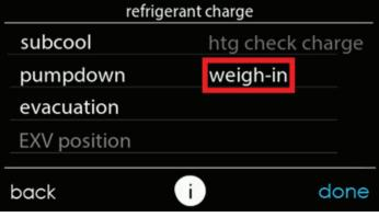
Fig. 16 – Weigh-in Option for charging below 65°F OAT and above 105°F OAT
