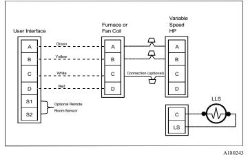
Fig. 4 – Liquid Line Solenoid Electrical Connection (Required for long line applications)
