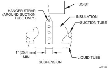
Fig. 1 – Connecting Tubing Installation
