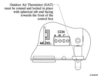
Fig. 29 – Outdoor Air Thermistor Mounting Location
