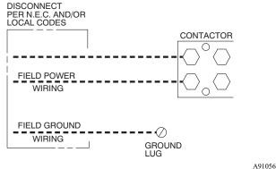
Fig. 9 – Line Power Connections
