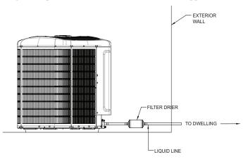
Fig. 7 – Liquid-Line Filter Drier for 5 Ton Applications
