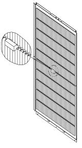
**Fig. 2 – Louver Spacer Location**
