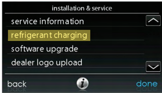
Fig. 11 - Select Refrigerant Charging
